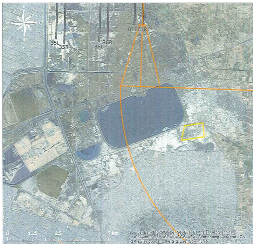
Figure 24. Conventional Departure Procedure to Runway 19L (Option 4.2)
