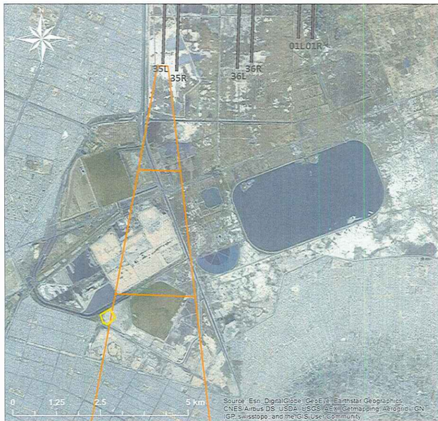
Figure 37. ICAO Annex 14 Approach Surface to Runway 35L (Option 5)
