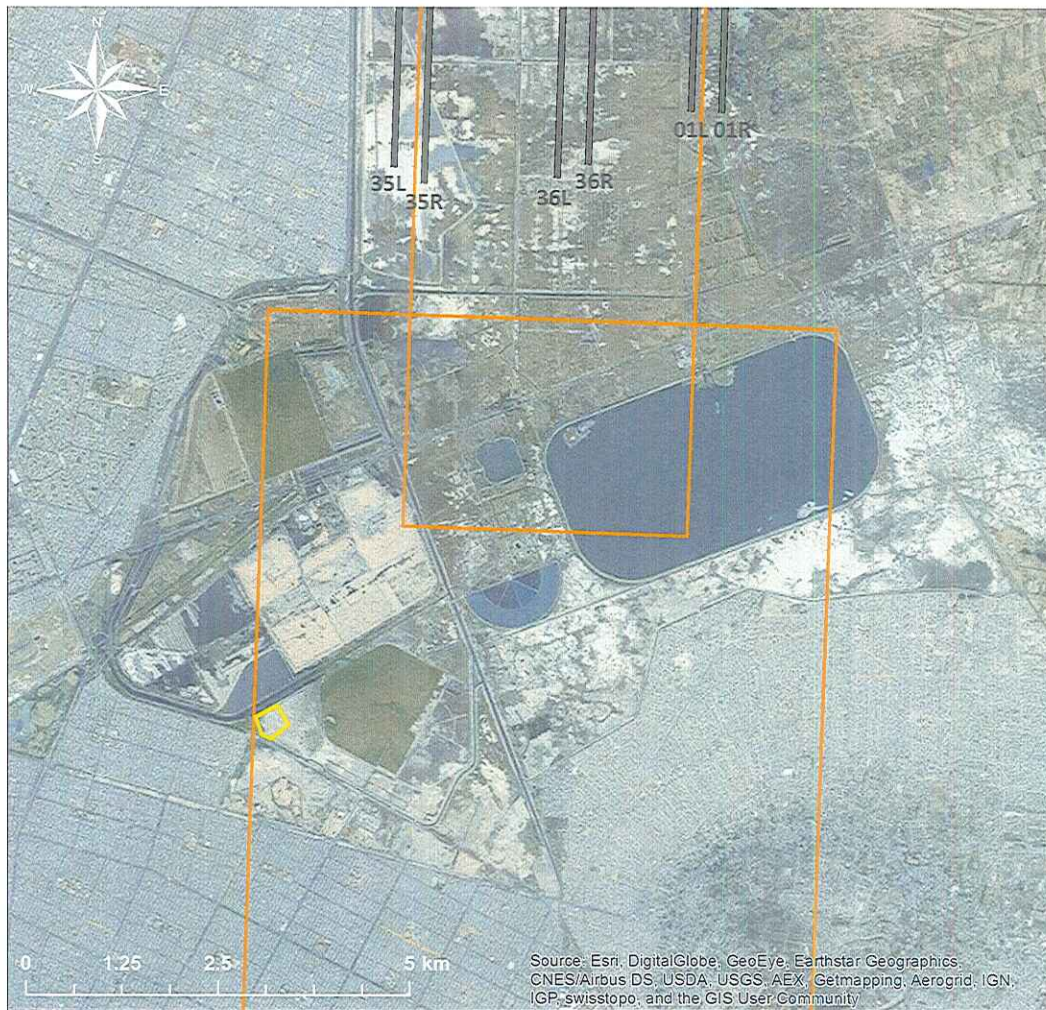
Figure 32. RNP AR Missed Approach Procedure for Runway 18R (Option 5)
