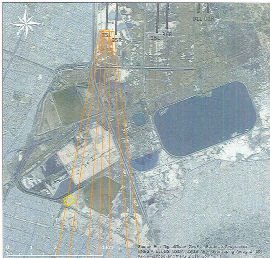
Figure 30. ILS CAT I/II/III Approach Procedure to Runway 35L (Option 5)
