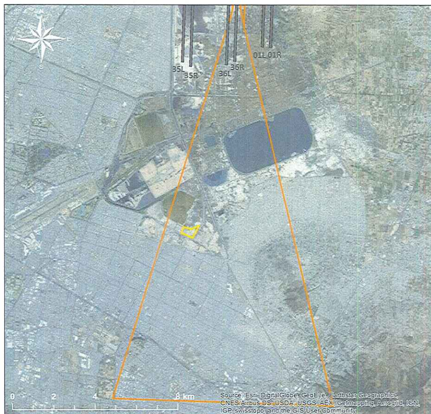
Figure 5. ILS CAT II/III Missed Approach Procedure for Runway 18L (Option 3)
