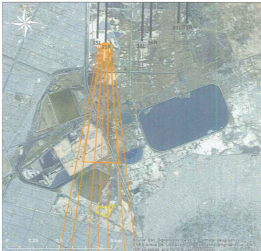
Figure 3. ILS CAT I/II/III Approach Procedure to Runway 35R (Option 3)
