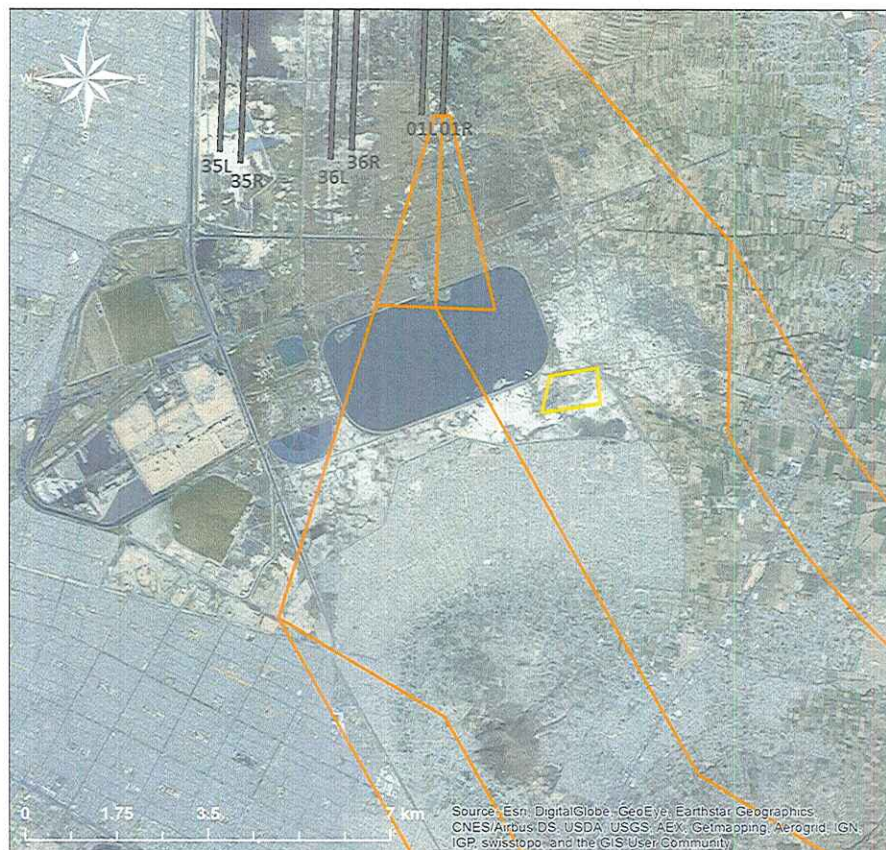
Figure 25. RNAV Departure Procedure from Runway 19L (Option 4.2)
