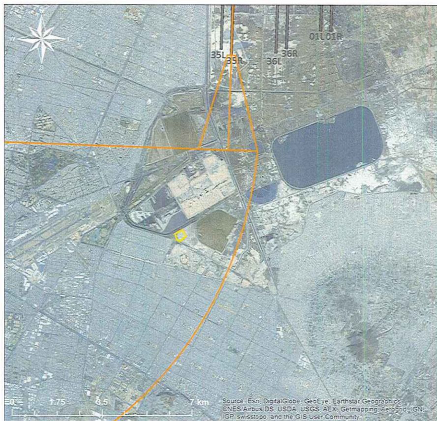
Figure 33. Conventional Departure Procedure from Runway 17L (Option 5)
