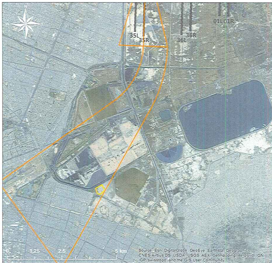
Figure 31. ILS CAT II/III Missed Approach Procedure for Runway 17L (Option 5)
