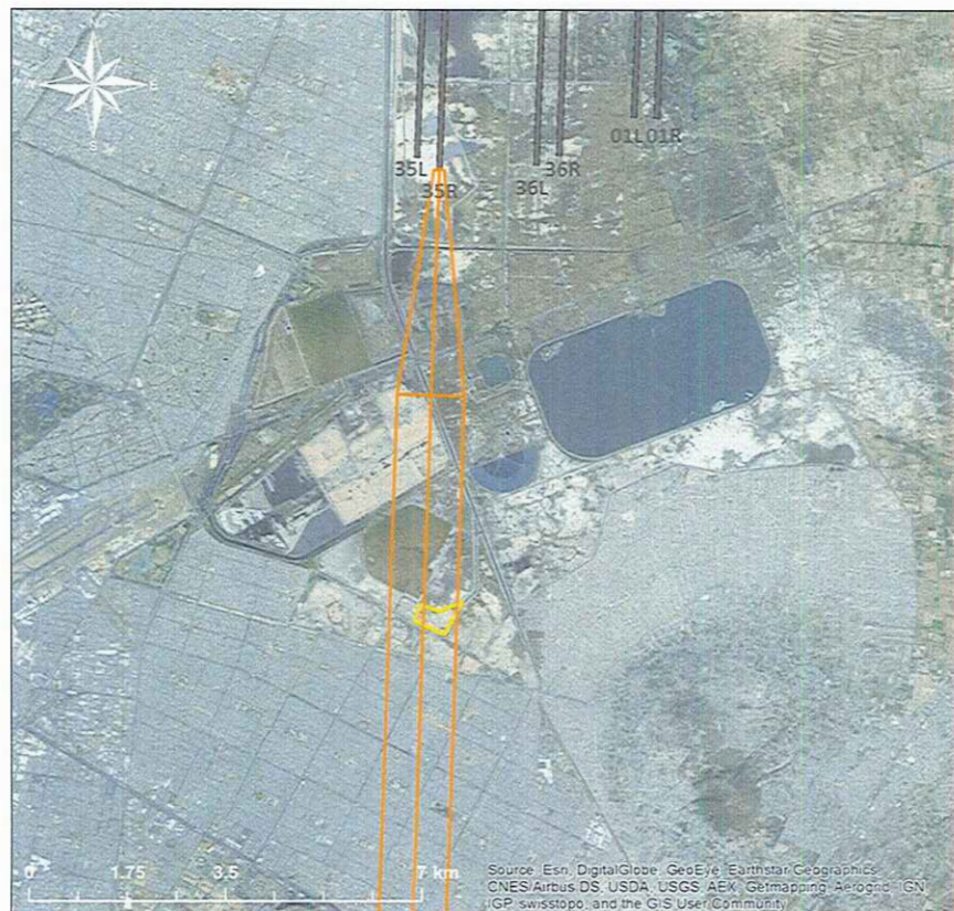
Figure 9. OEI Procedure for Runway 17L (Option 3)
