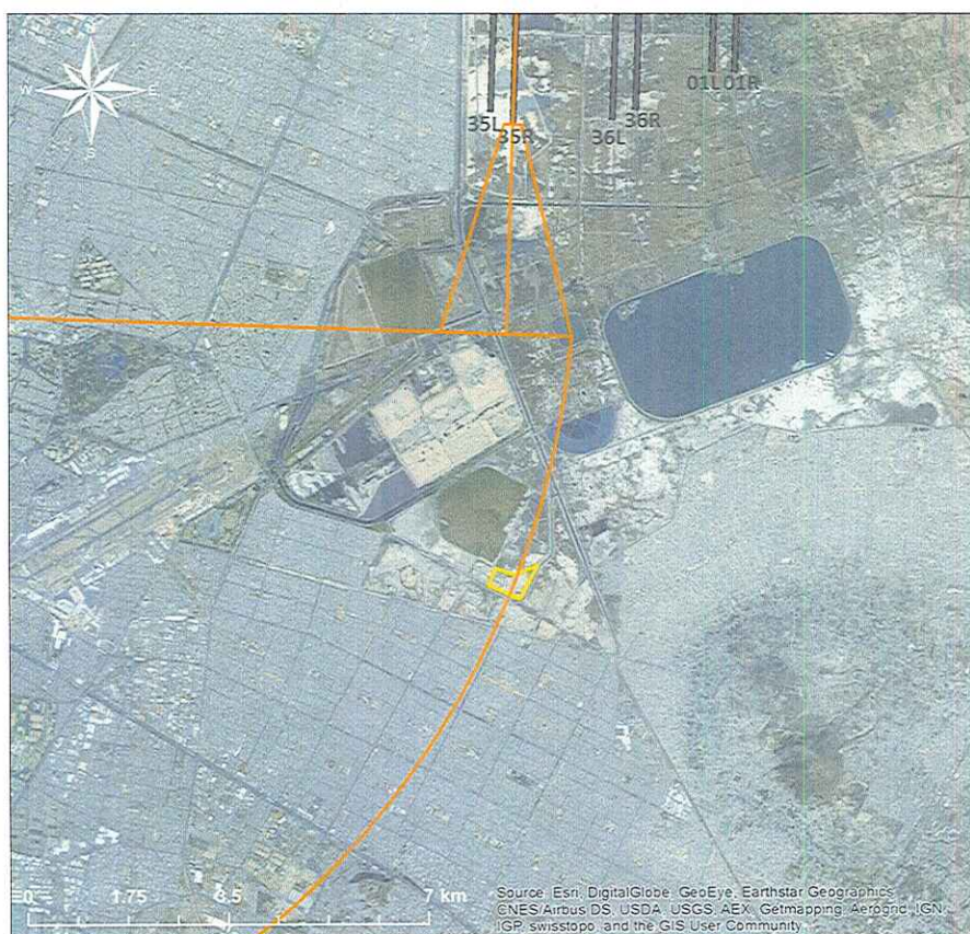
Figure 7. Southbound Conventional Departure Procedure from Runway 17L (Option 3)
