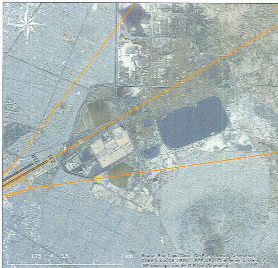
Figure 35. ILS CAT I Missed Approach Procedure (Option 5)
