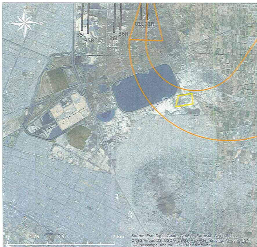
Figure 22. ILS CAT II/III Missed Approach Procedure for Runway 19L (Option 4.2)
